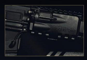
The control cable connects the lower to the upper receiver and is designed so that the upper can be separated from the lower at the rear take down pin without having to remove the cable.
